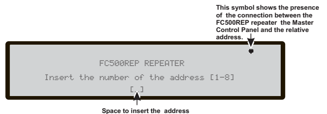
Figure 50 Display to insert a new FC500REP address
