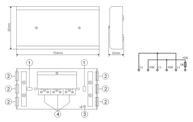
Fig.1. The junction box and wiring diagram.
