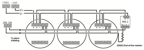
Figure 2-15 Smoke Detector Wiring
