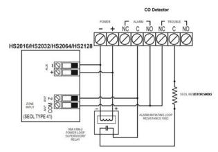
Figure 2-17 CO Detector Wiring
