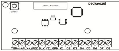
Figure 2-5 HSM2208 Output Expander
